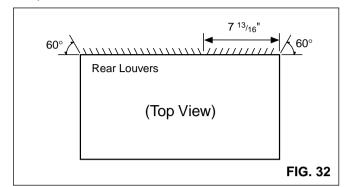
2 If the wall sleeve already has a rear grille, skip to step 4. If the wall sleeve does not have a rear grille or louvered panel, install the plastic grille from the kit. Cut the plastic grille to 26-1/2" wide and 15-1/2" high. Place the plastic grille to the inside of the wall sleeve at the rear flange.
